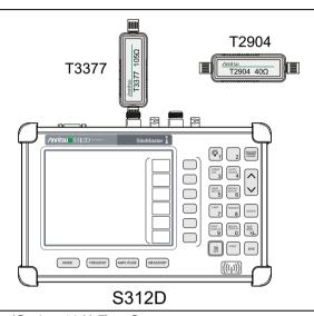
Figure 2-12. Bias Tee Verification (Option 10A) Test Setup
