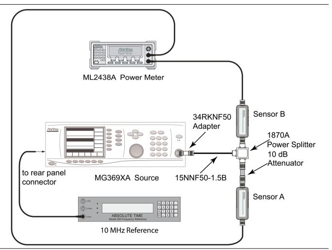
Figure 2-6. Spectrum Analyzer Level Accuracy Verification Characterization Setup
