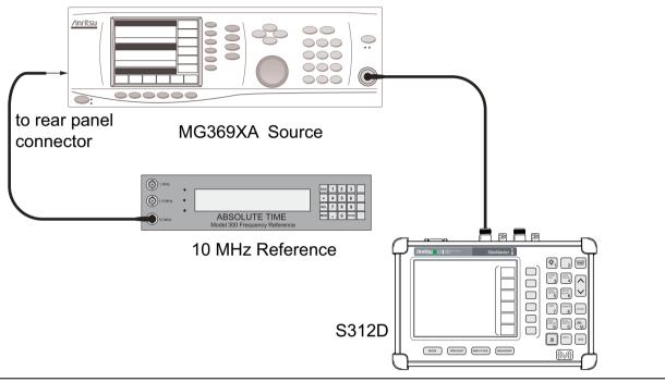
Figure 2-4. Spectrum Analyzer Frequency Accuracy Test Setup
