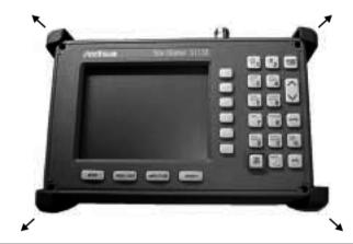
Figure 3-3. Removing the Corner Bumpers
