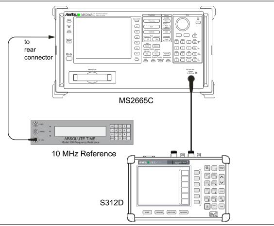
Figure 2-1. VNA Frequency Accuracy Test Setup
