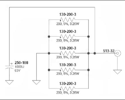
Figure B-1. Anritsu Model T2904 High Current Test Fixture (for Option 10A)
