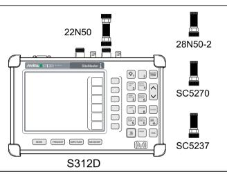
Figure 2-2. VNA Return Loss Verification Test Setup
