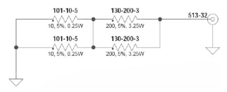
Figure B-2. Anritsu Model T3377 Low Current Test Fixture (for Option 10A)
