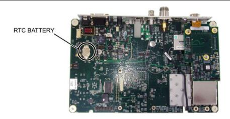
Figure 3-6. RTC Battery Location
