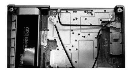
Figure 3-5. S312D Spectrum Analyzer PCB
