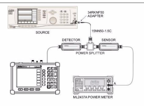
Figure 2-11. Power Monitor Verification (Option 5) Test Setup
