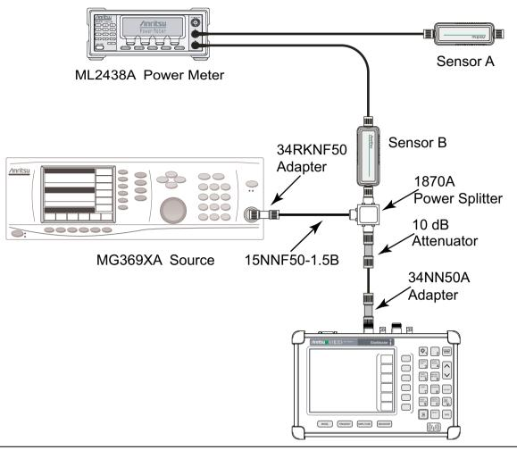
Figure 2-14. Power Meter Verification (Option 29) Test Setup
