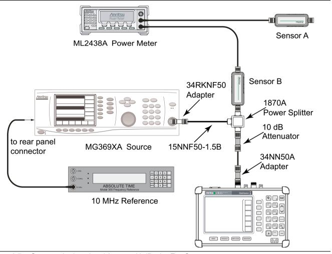
Figure 2-7. Spectrum Analyzer Level Accuracy Verification Test Setup
