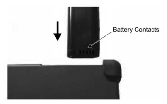
Figure 3-2. Battery Pack Replacement
