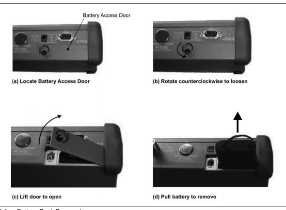
Figure 3-1. Battery Pack Removal
