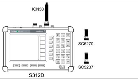
Figure 2-3. InstaCal Module Verification Test Setup
