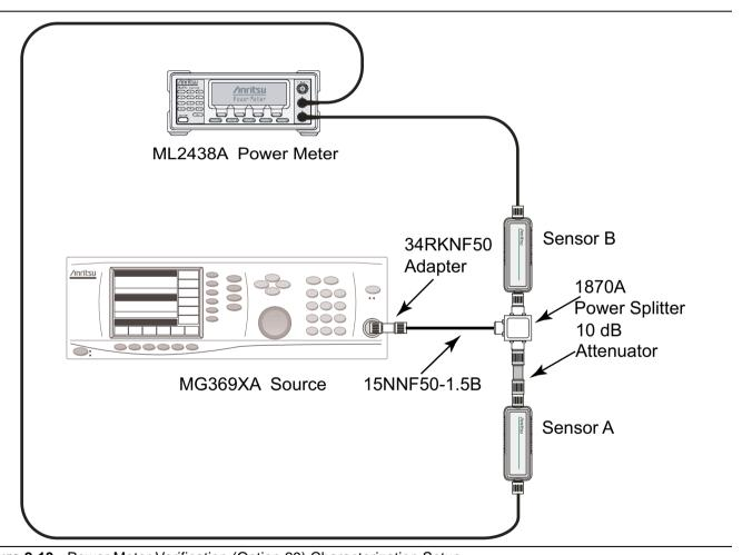
Figure 2-13. Power Meter Verification (Option 29) Characterization Setup
