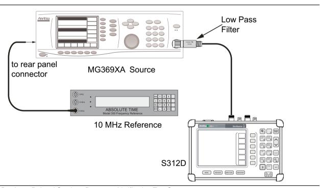
Figure 2-5. Input Related Spurious Response Verification Test Setup
