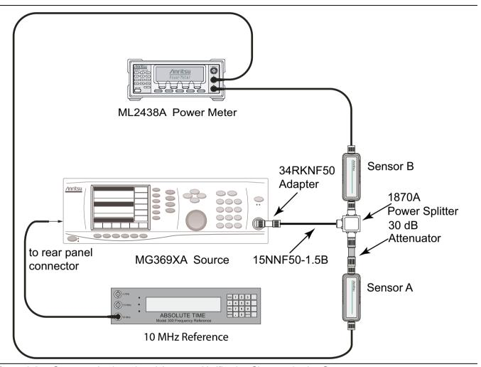
Figure 2-8. Spectrum Analyzer Level Accuracy Verification Characterization Setup
